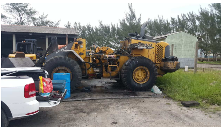
Figura: 14: Cabine removida, Autor (2020).
