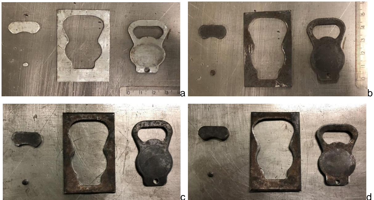
Figura 29 – Teste em chapa de 1,5mm (a), 2,0mm (b), 2,5mm (c), 3,0mm (d).
